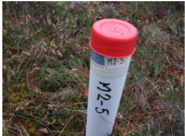
Groundwater monitoring well in Melnais Lake Mire. Photo: Persijs Gederts
