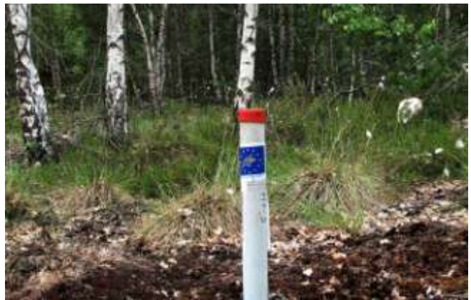
Hydrological monitoring well in the project sites.
