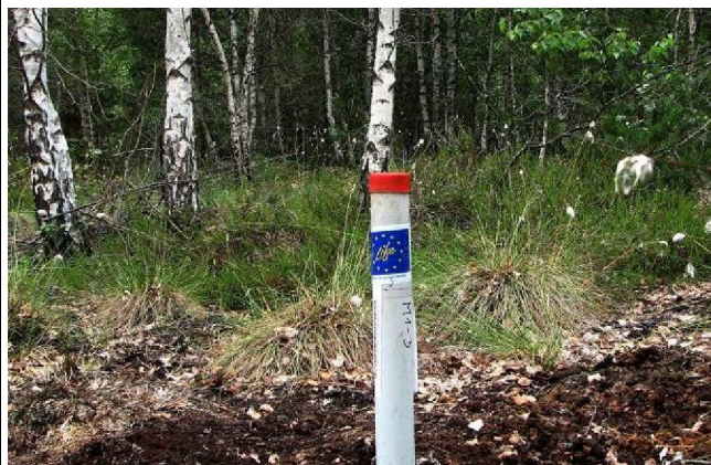
Hydrological monitoring wells in the project sites. Photo: G. Balodis
